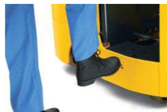
Travel and lifting are stopped when the operators leaves the compartment
