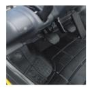
The wide, flat floor accommodates the tilt cylinder under the floor. Suspended (type) pedals are used to provide extra foot space, which significantly reduces operator fatique. The new wide-open, non-slip step and spoon-curved fender makes getting in and out easy and safe.
