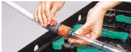
Start of water refilling: Opening the faucet automatically starts refilling water into all batteries (be sure to open the faucet fully).
